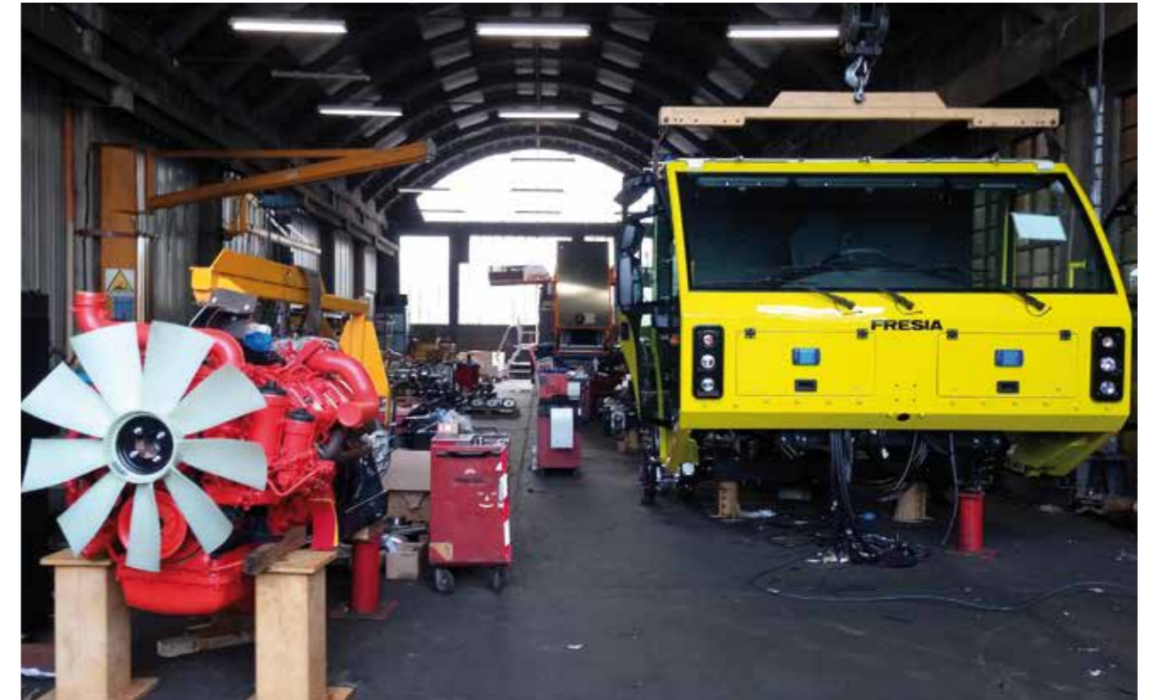
A colourful collaboration. The red Scania DC16 engine, to the left, is ready to be mounted on a yellow Fresia crash tender chassis. For this type of special vehicles, acceleration, performance and reliability are key issues
