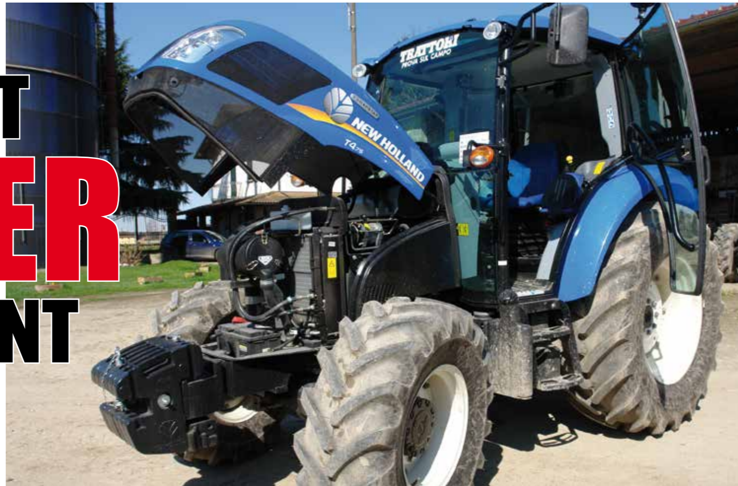
Even in this power range, 3 and 4 cylinder diesel engines just below 56 kilowatts, DOC and DPF are an extremely common choice...
